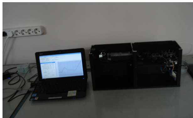
Figure 1. A combined Led spectrophotometer and spectroellipsometer.
