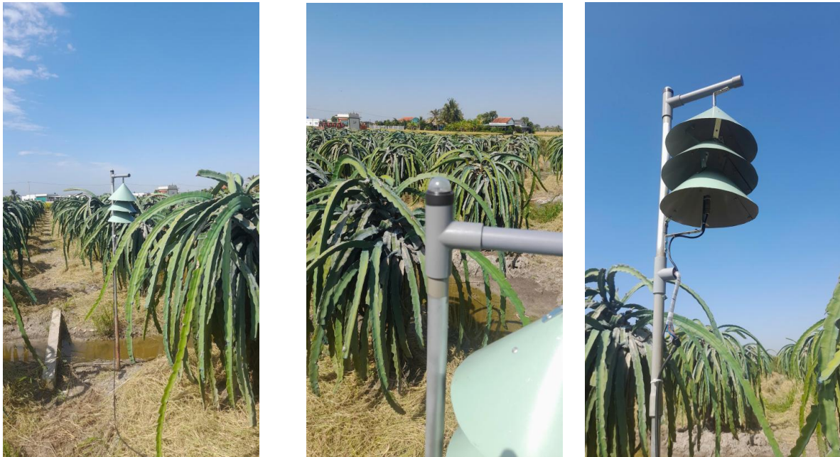
(a) Sensors installed in the dragon fruit farm. (b) Light intensity sensor. (c) Temperature and humidity sensor.
