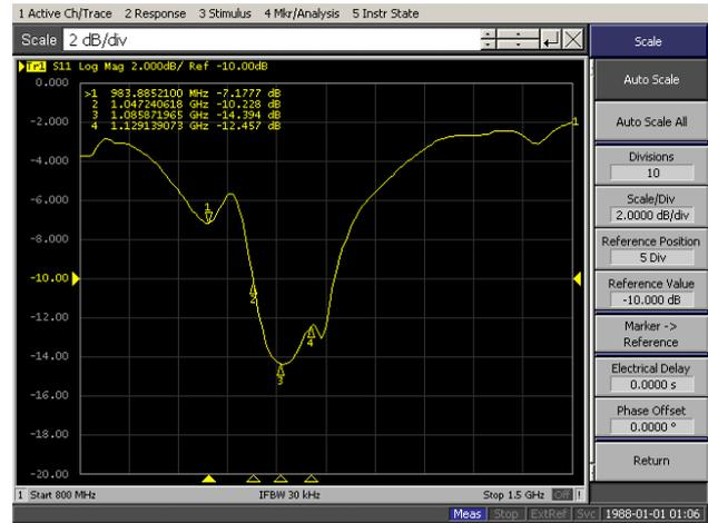
Figure 12. S11-value of the proposed tag antenna with L1 at 13.4 nH
