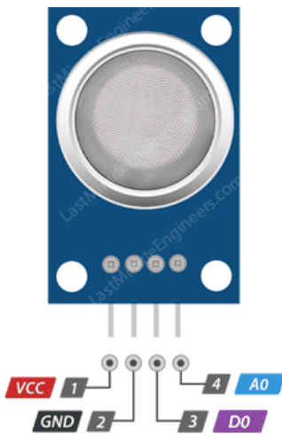
Figure 3. The sensor MQ 2 pinout [23].
