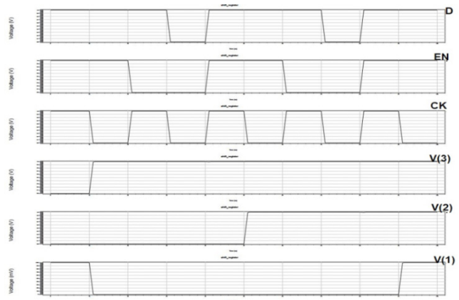
Figure 12. Waveforms of three-bit shift register.
