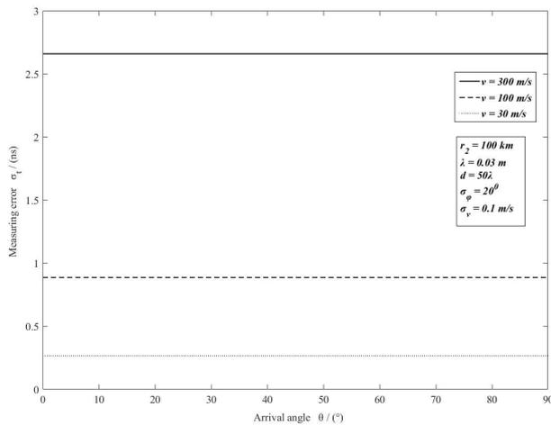
Figure 12. The measurement error at different flight speeds
