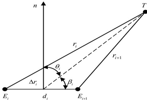
Figure 2. Schematic diagram of single base array
