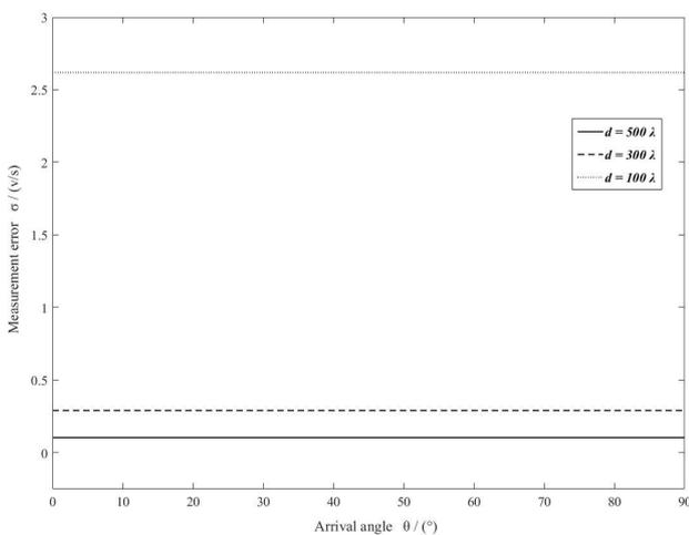
Figure 9. Measurement error at different baseline lengths
