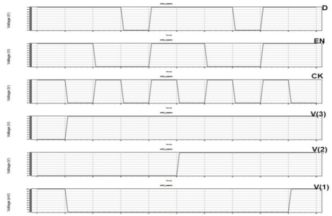
Figure 12. Waveforms of three-bit shift register.
