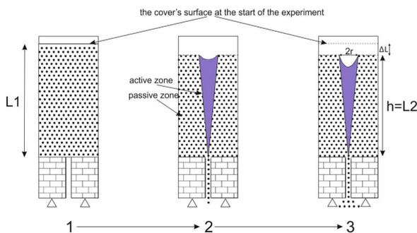
**Figure 4.** Flowchart of the depression's developing. 1. the start of the experiment, 2. the matter sheds through the chimney, 3. a depression formed on the cover at the end of the experiment, L1. thickness of the cover before the experiment, h=L2. thickness of the cover after the experiment, 2r. diameter of the depression,  $\Delta L$  subsidence of the cover's surface
