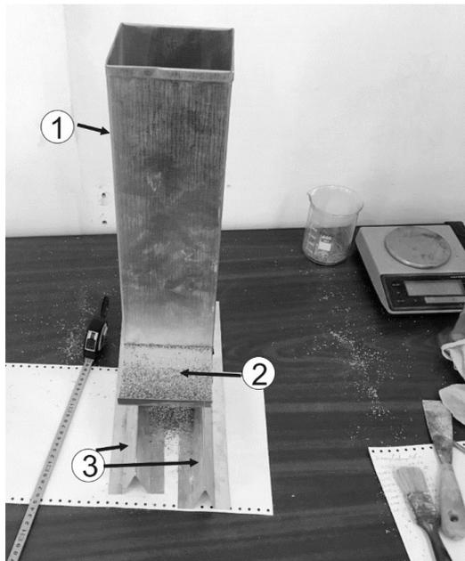
**Figure 1.** The experimental tool and its parts, 1. the metal prism, 2. the metal plate what separates the drilled plaster block and the cover, 3. metal rails which create the void space below the tool
