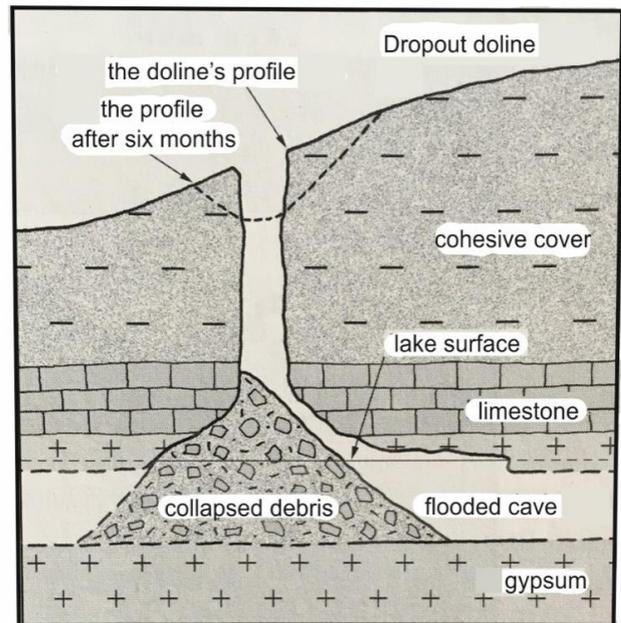
**Figure 2.** Horizontal cave system under a dropout doline [16]
