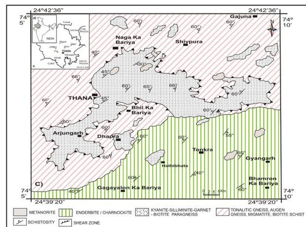
**Figure 1.** Geological map around Thana, Bhilwara, Rajasthan by author <sup>[1]</sup>, showing distribution of different litho units
