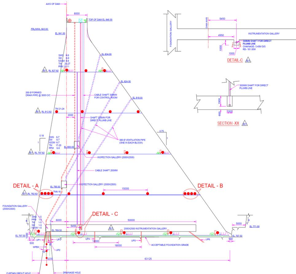
Figure 7. Maximum non-overflow section showing location of different instruments at PHEP-II dam (Ref: CWC/INST/PNSC-9810-C-2131(R1)) [7]
