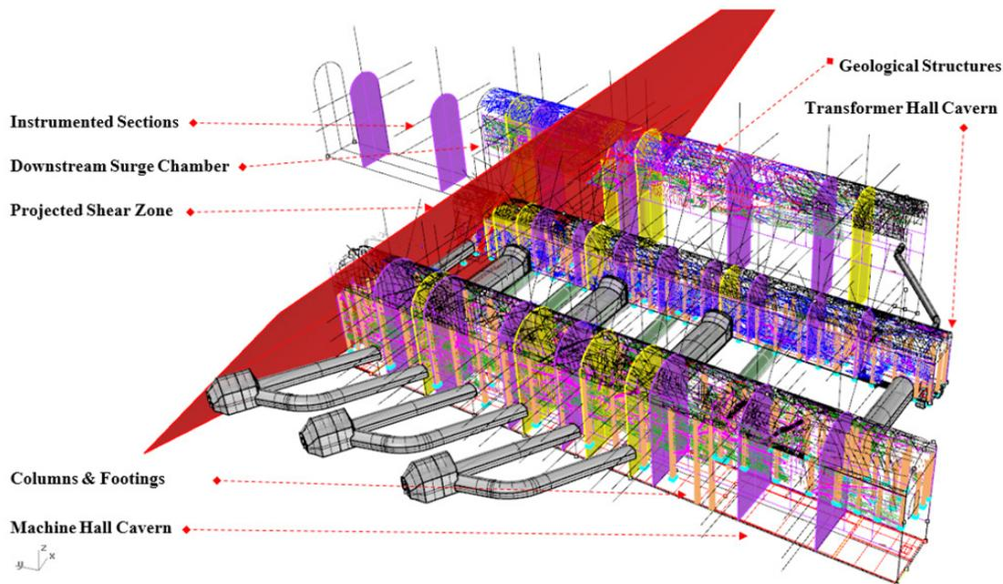
**Figure 8.** 3-D view of PHC incorporating actual coordinates, civil structures, geological structures and instrumentation layouts (Ref: 3D Instrumentation Model by NIRM) <sup>[1][5][8]</sup>
