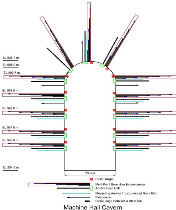
**Figure 9.** Section showing the location of different instruments in Machine Hall Cavern, PHEP-II <sup>[1][5][8]</sup>
