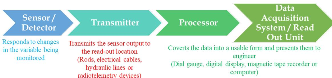
Figure 2. Components of an instrument
