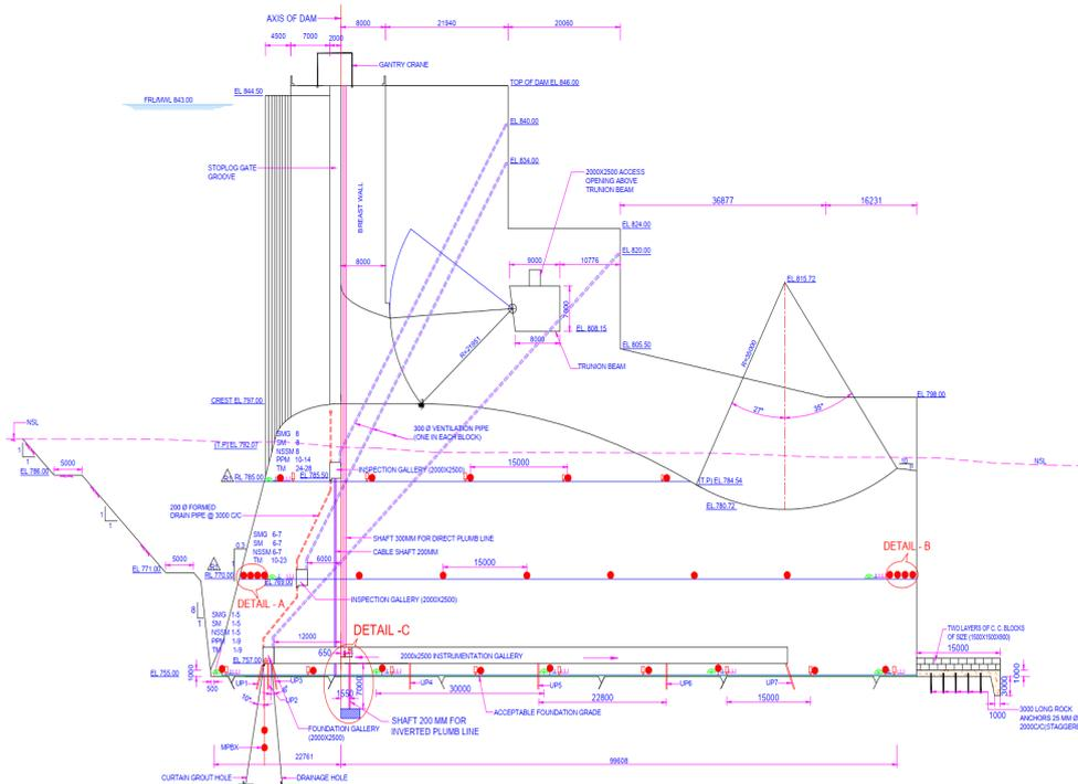
Figure 6. Maximum sluice section showing location of different instruments at PHEP-II dam (Ref: CWC/INST/PNSC-9810-C-2130(R1)) [7]
