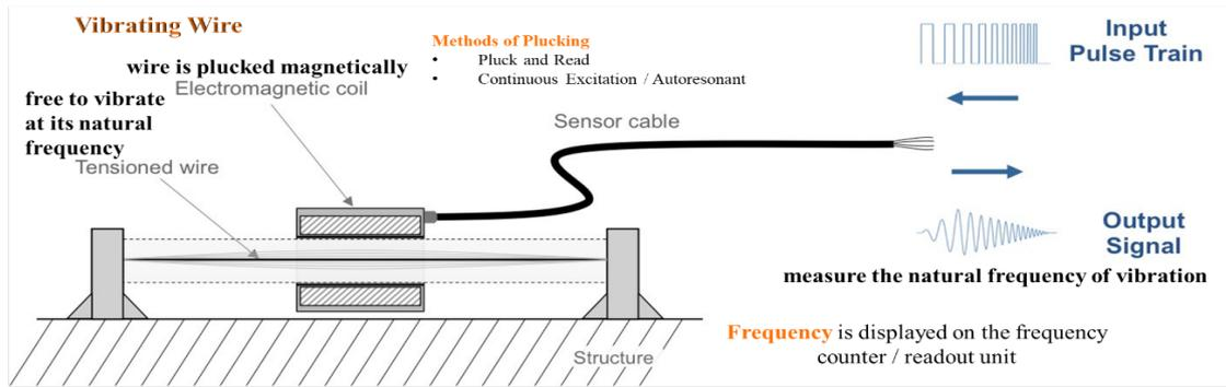
Calibration curve or table or linearizing circuit through **gage factors** are used for calculating desired parameter from change in frequency.
