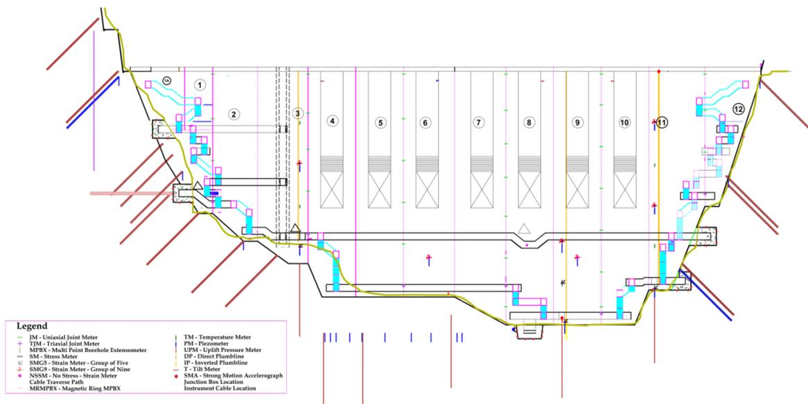
Figure 5. Longitudinal section at dam axis showing location of different instruments at PHEP-II dam (Ref: CWC/INST/PNSC-9810-C-2132(R1)) [7]
