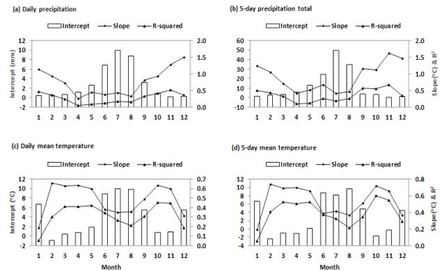
**Figure 5.** The regression models by months with the Khanchikot temperature/ precipitation as the dependent variable and the Taulihawa as independent variables. Regression models using the daily (a) and 5-day (b) mean temperature data, and daily (c) and 5-day (d) total precipitation data
