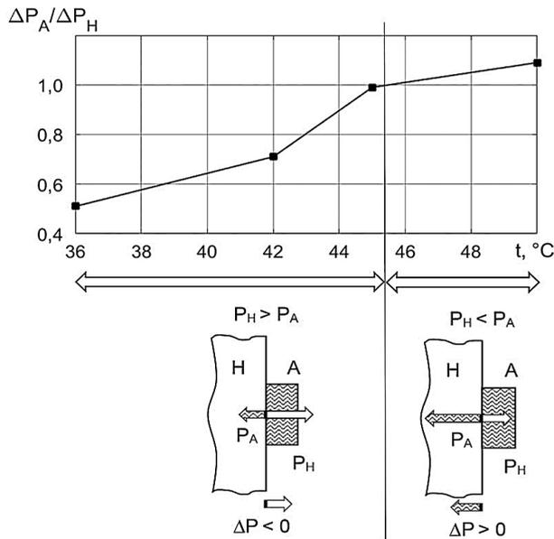
**Figure 4.** Dependence of relative power on temperature and distribution of electromagnetic energy flow for ozokerite applicator during cooling
