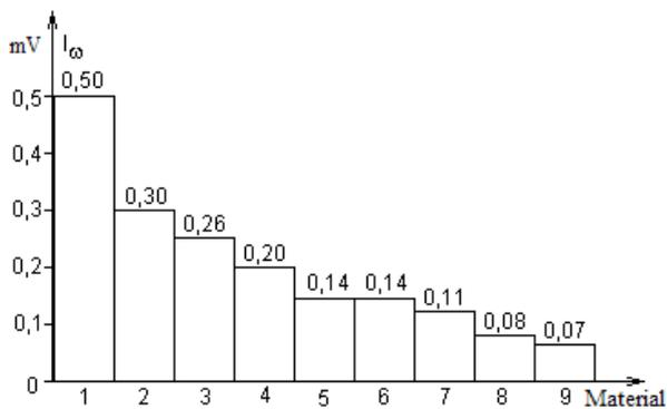
Figure 12. Distribution emissivity of textile materials for clothes
