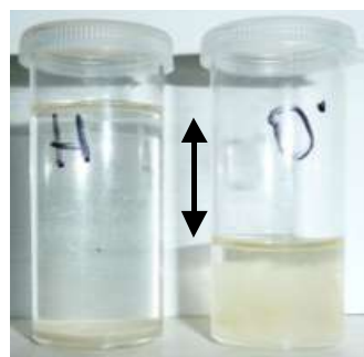
Figure 4. There is a swelling of starch in water with a different electric potential. Starch does not swell in water with the potential of -250 (left) and swells in water with the potential of +250 \text{ mV} (right)
