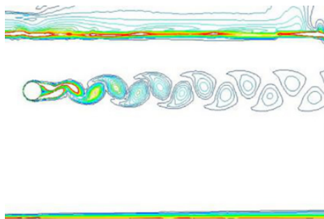
Figure 6(c). Vorticity magnitude of the cylinder for H/D=3
