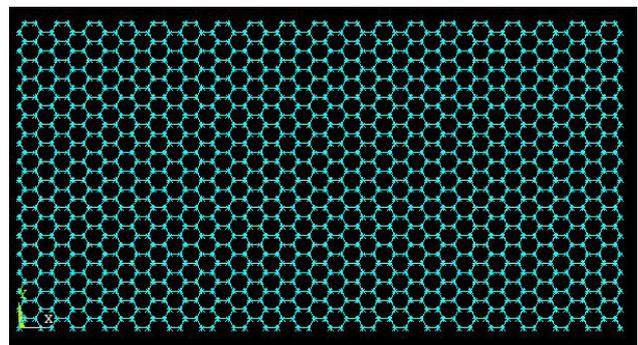
**Figure 7.** Space Frame of (19, 19) configuration
