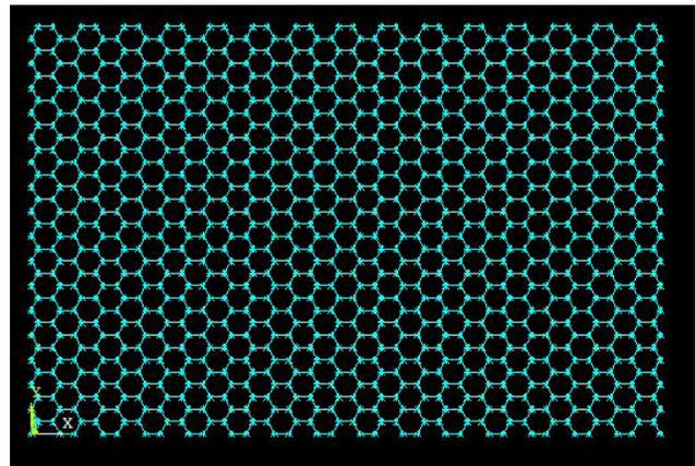
**Figure 6.** Space Frame of (15, 15) configuration
