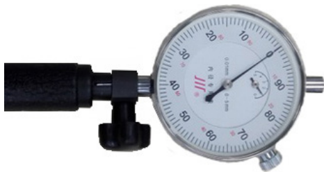
Figure 4. Percentimeter status after calibration of internal diameter scale
