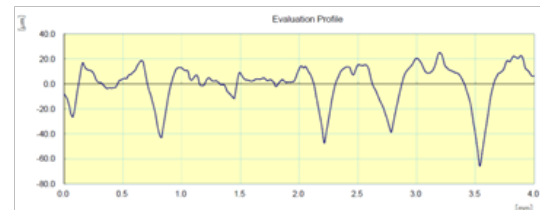
(c) Surface Roughness plot before chemical vaporization
