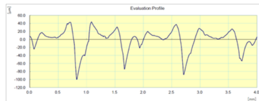
(c) Surface Roughness plot before chemical vaporization
