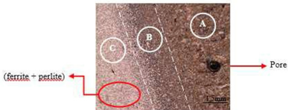
Figure 10. Micrograph of the welded joint at 50x magnification
