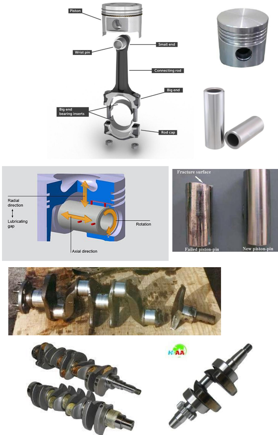
Figure 1. Individual components of the assembly, including piston, connecting rod, pin, and crankshaft
