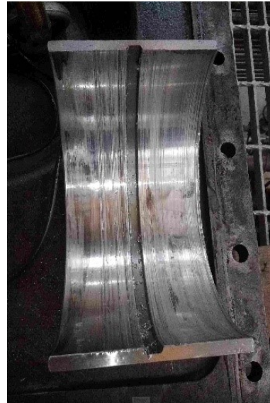
Figure 5. Wear status of aircraft bearing bushing.
