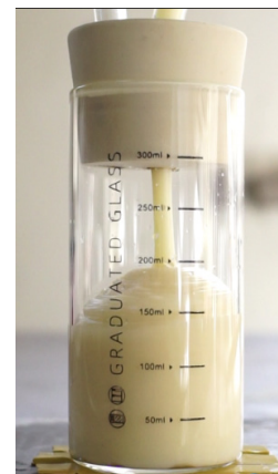
Figure 3. The vacuum filling with hair conditioner.
