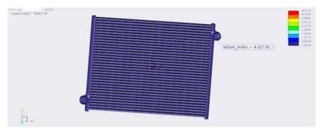
Figure 5. Failure index distribution of the Tresca theory for the thermal analysis
