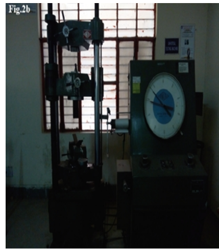
Figure 2b. Universal testing machine for tensile testing
