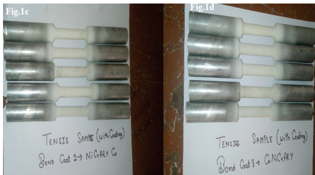
Figure 1 c. NiCoCrAlY bond coated TBC sample.
