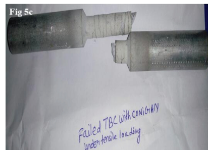
Figure 5. Failed TBC sample under tensile loading for: (a) NiCoCrAlY, (b) CoNiCrAlY Bond coat.
