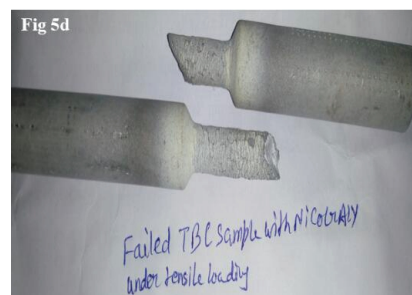
Figure 5. Failed TBC sample under tensile loading for: (c) NiCoCrAlY, (d) CoNiCrAlY Bond Coat.
