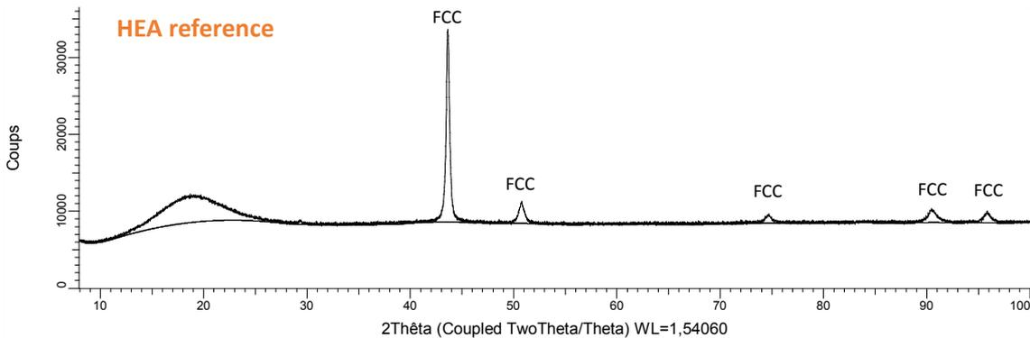
**Figure 1.** Diffractogram of the HEA reference alloy
