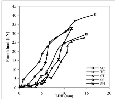
**Figure 6.** Punch load and limiting dome height diagram for welded blanks made with different tool pin profiles
