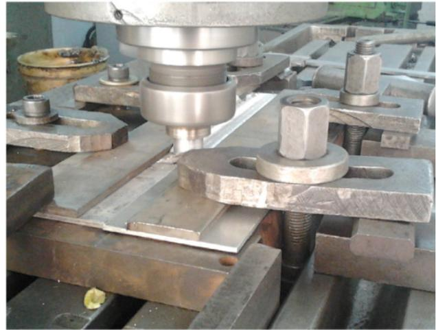
**Figure 1.** FSW arrangement
