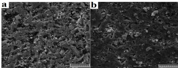
**Figure 7.** SEM micrographs for (a) AA6061 (b) AA2014 base materials
