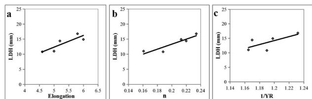
Figure 5. Variations of LDH for (a) elongation (b) strain hardening component (c) work hardening capacity of welded blanks
