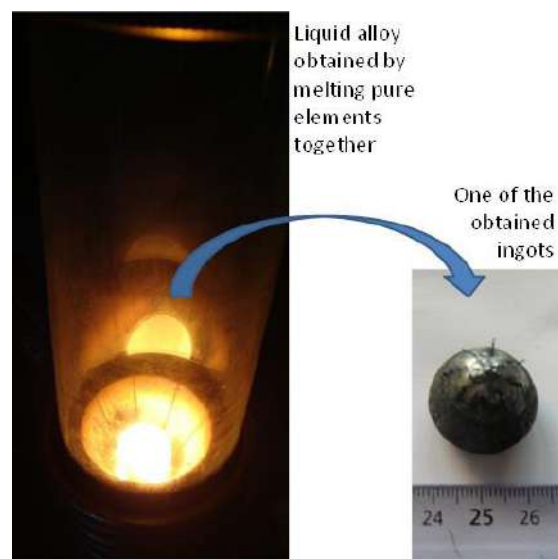
Figure 2. Illustration of the elaboration of the alloys for the study (high frequency induction melting and solidification in a cooled copper crucible)
