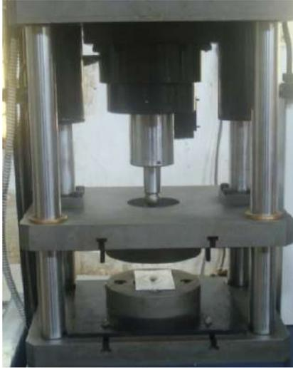
**Figure 3.** Arrangement of hydraulic press with punch, dies and welded blank
