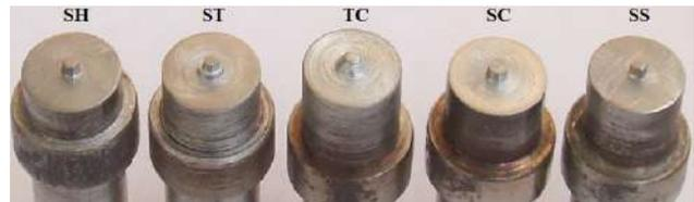
Figure 2. Photograph of different tool pin profiles
