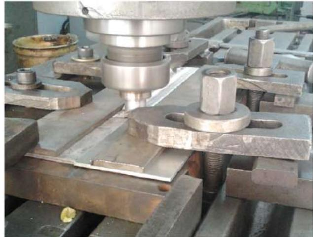
Figure 1. FSW arrangement
