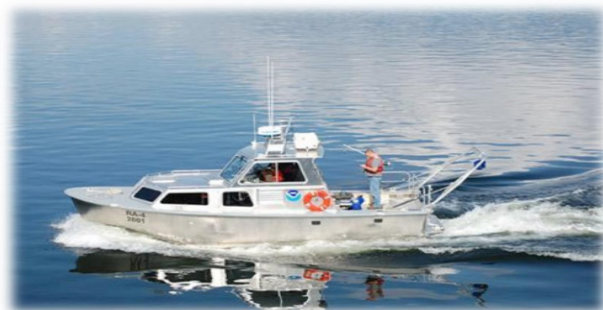
A typical small hydrographic launch used for near-shore and harbour surveys
