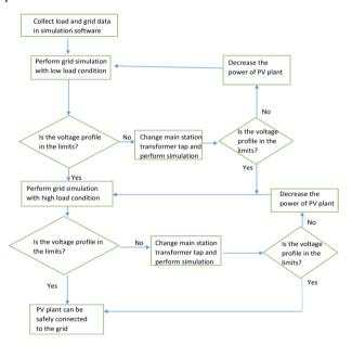
Figure 6. proposed algorithm for PV plant connection with considering voltage limitations
