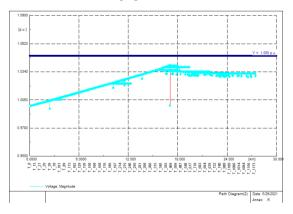
**Figure 2.** voltage profile of feeder 1 in presence of PV plant in low load condition
