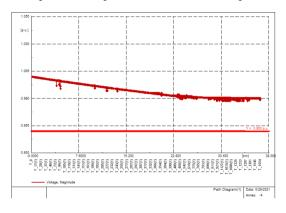
Figure 3. voltage profile of feeder 2 in low load conditions
