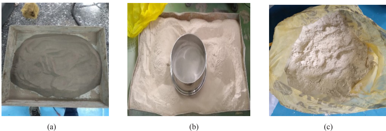
Figure 1. Materials used in the Study (a) soil, (b) BWIA and (c) lime
