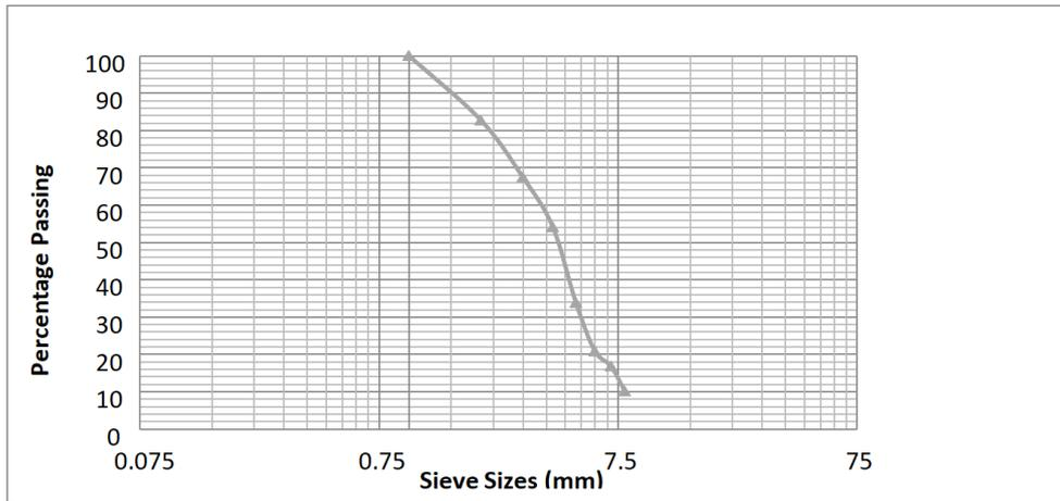
Figure 2. Variation of % Passing with sieve sizes for coarse aggregate
