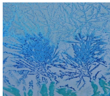
Figure 3. The crystals formed after drying an aqueous solution of \text{CuCl}_2 , which was previously subjected to the action of EMF, pulsing with a frequency of 10 Hz for 10 minutes; to increase the contrast, the crystals were treated with ammonia vapor [3]
