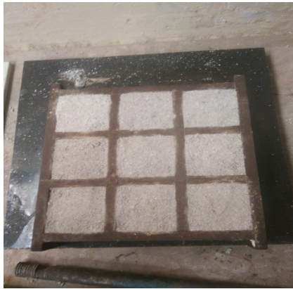
Figure 4. Finished Lime Mortar
