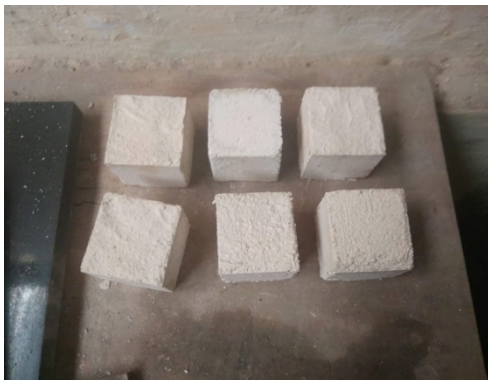
Figure 5. Demoulding and kept For Curing
