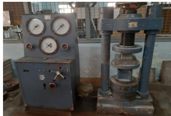
Figure 6. Compressive Strength Testing Equipment
