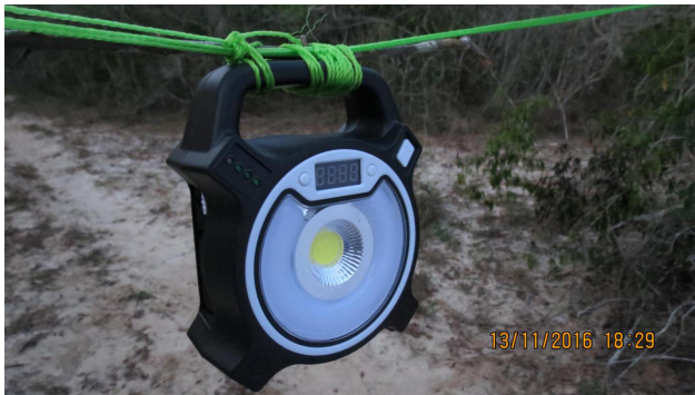
Figure 2. A mounted solar light and battery (DP Light DP-6005A) which was used to attract air-borne invertebrates active at night.
