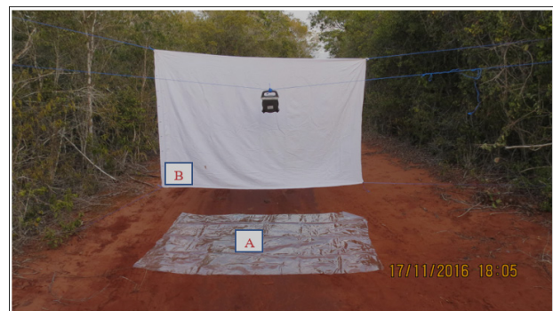
Figure 3. The operational set up of solar light trap and battery (DP Light DP-6005A) with a transparent plastic sheeting spread on the ground (A) and suspended white cloth screen (B) for invertebrates landing
