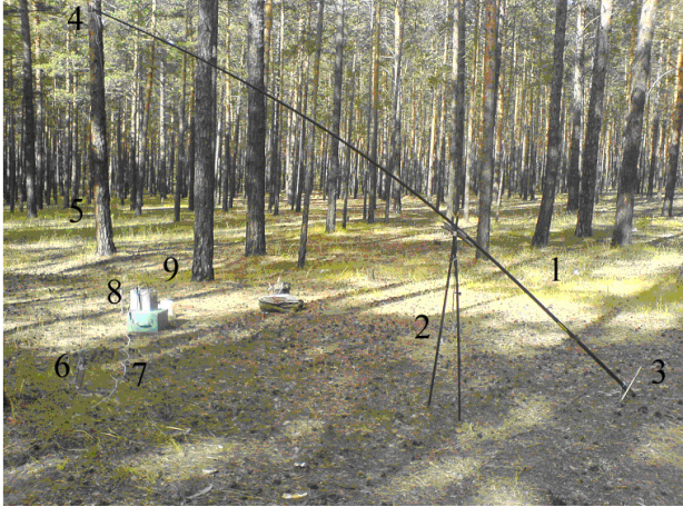
Figure 4. Modified IPI-300 kit for measuring the electro-physical characteristics of the forest media. Vertical orientation of the electric antenna. 1. Telescopic rod; 2. Rod support; 3. Bottom mount; 4. Electric antenna suspension; 5. Dipole Nadeenko; 6. Input antenna amplifier; 7. Shielded wire; 8. Magnetic antenna; 9. MSI-300.
