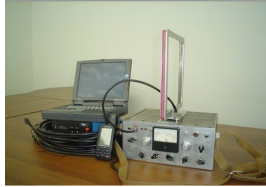
Figure 2. Surface impedance meter kit (MSI-300). The number 300 indicates the measuring range in kHz. A reeled insulated cable and frame are shown.
