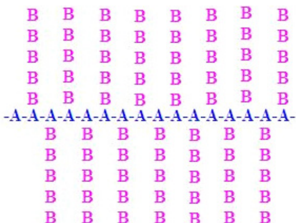
Figure 2. Schematic diagram of graft copolymers
