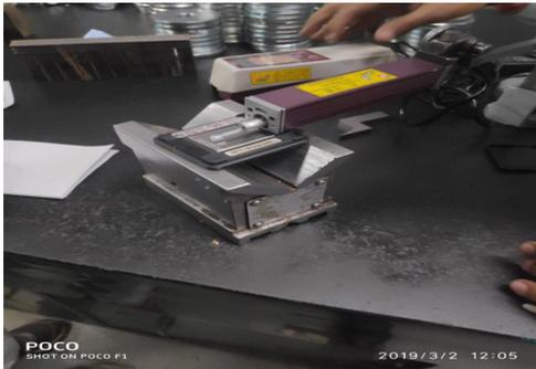
Figure 9. Surface Tester used in present study
