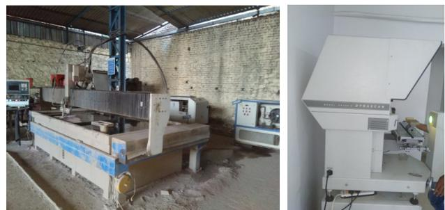
Figure 6. KMT abrasive water jet machine and profile projector used in the present study
