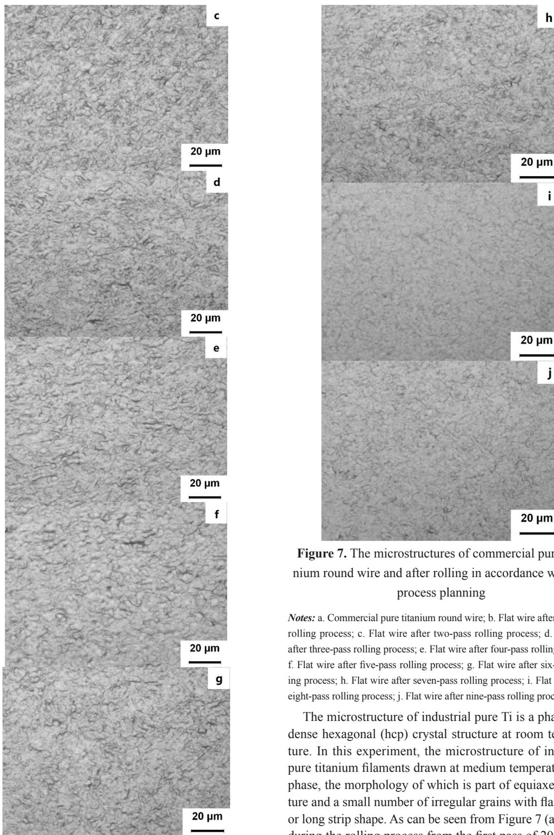
**Figure 7.** The microstructures of commercial pure titanium round wire and after rolling in accordance with the process planning
