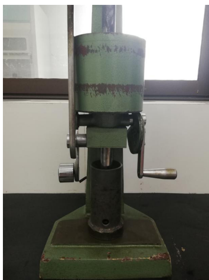
Figure 2. The equipment for measuring the flowability of the coated sand
