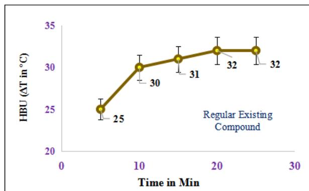
**Figure 7.** Heat Buildup of Regular Existing Compound Heat Buildup decrease in percentage (%) than Regular Existing Compounds.
