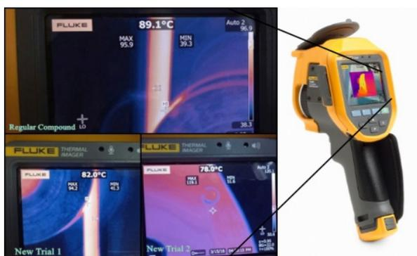
**Figure 22.** Belt Temperature Study by IR Thermal Imager
