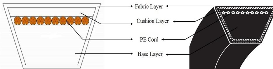
Figure 2. Cross-section of a Transmission V-Belt
