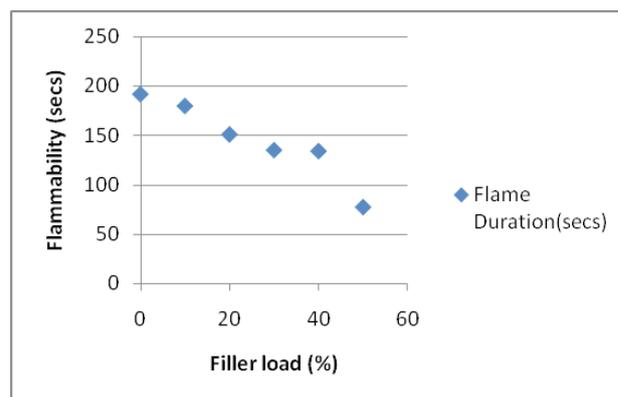
**Figure 5.** Effect of filler load on flammability.
