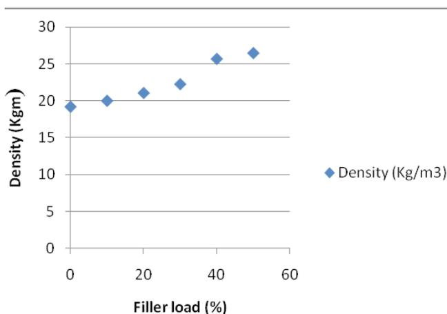
**Figure 1.** Effect of filler load on Density.
