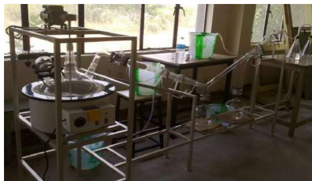
Figure 3. Waste bio-plastics to fuel production through de-polymerization
