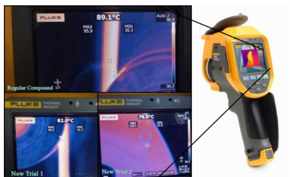
Figure 22. Belt Temperature Study by IR Thermal Imager
