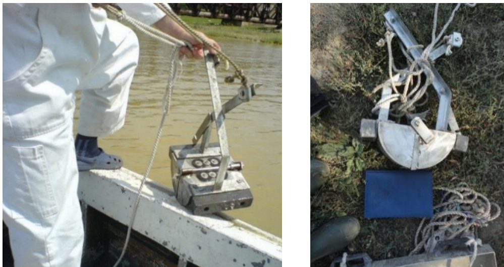
Figure 1. Van Veen Bodengraifer.
