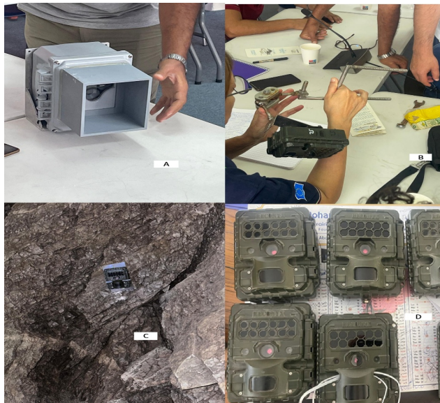
Figure 3. Camera-Trap Equipment and Deployment Process in the Al Hoceima Marine Protected Area (MPA). (a) RECONYX infrared camera traps prepared for deployment, configured with motion-activated sensors and powered by lithium batteries to ensure prolonged operation in humid cave environments; (b) Custom-designed protective casing engineered to shield units from moisture, debris, and direct wave exposure inside sea caves; (c) Field testing of the stainless-steel mounting bracket system, allowing flexible orientation and secure anchoring of cameras to irregular rock surfaces; (d) Final installation of a camera trap inside a high-priority Category A cave, positioned on an elevated rock wall facing the internal haul-out platform to optimize monitoring coverage.
