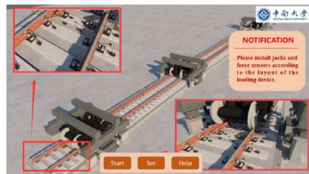
Figure 3. Demonstration of the experiment process of crawling and off-axis impact of large-scale turnouts in subway
