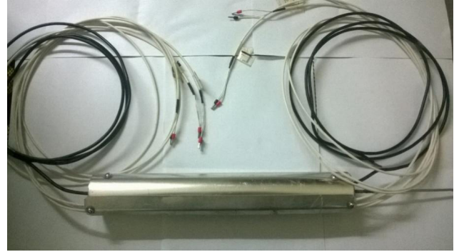
Figure 2. Aluminum thin cylinder having five thermocouples at the inner surface
