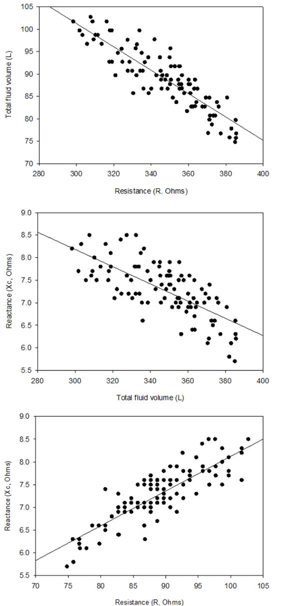
**Figure 6.** Top panel: the relationship between resistance (R) and total body water (TBW):  $R = 179.5 - TBW \times 0.261$ ;  $r^2 = 0.787$ ;  $p < 0.001$ . Middle panel: the relationship between reactance (Xc) and TBW:  $Xc = 13.92 - TBW \times 0.0191$ ;  $r^2 = 0.524$ ;  $P < 0.001$ . Bottom panel: the relationship between reactance (Xc) and resistance (R) at the frequency of 50 kHz. Data from all horses at all time points.  $Xc = 0.490 + R \times 0.0763$ ;  $r^2 = 0.721$ ;  $P < 0.001$
